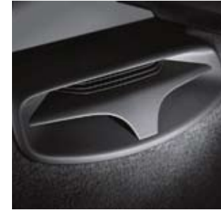
Active subwoofer, 10.2 cm x 15.3 cm bass speaker in the passenger footwell
